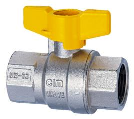
Manufactured according to management requirements of EN ISO 9001 standard. 100% tested in accordance with EN 12266-1 standard. Suitable for gas at low pressure, in detail: Natural gas: gas by-product of oil (methane); Town gas: manufactured through different processes (cracking - cokerie - etc.) Liquid gas: propane and mixture of propane/butane gas.
