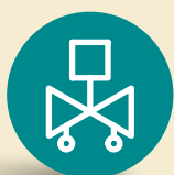
Válvula de equilibrio y control de orificio variable Variable orifice control and balancing valve
