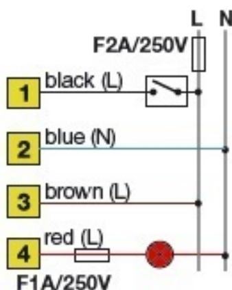
Connection with 3 cables SPDT
